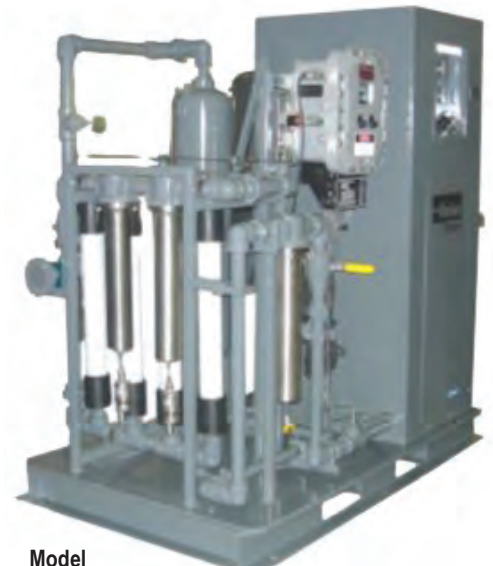
Model SMD-FB-1508-4 Gas Seal Unit with Membrane Dryer
