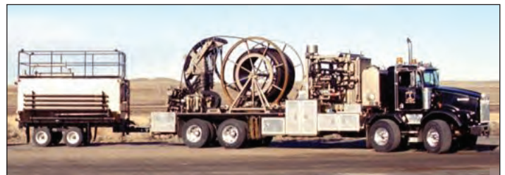
Typical Coiled Tubing Rig for Well Workovers
